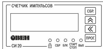
Figure 6.3 – Front panel of the device in housing for panel-mounting Щ2
